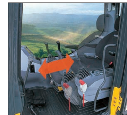
Seat Sliding Amount: 340 mm 13.4", increased 120 mm 4.7"
