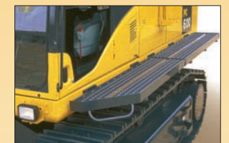
Large Handrail and Wide Catwalk
